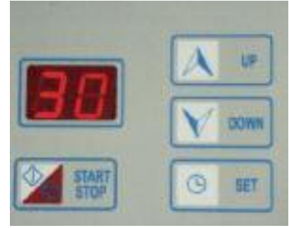
Fig. 21, 22, 23: The material should be handled according to the manufacturer's instructions. It is important to add exactly 5 drops of liquid into the powder capsule and allow it to mix at a speed of 4000 – 4200 rotations/min for 30 seconds.
