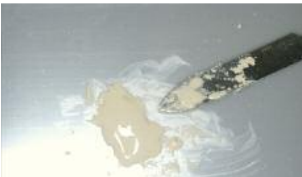
Fig. 24: Correctly mixed material must have a creamy consistency
